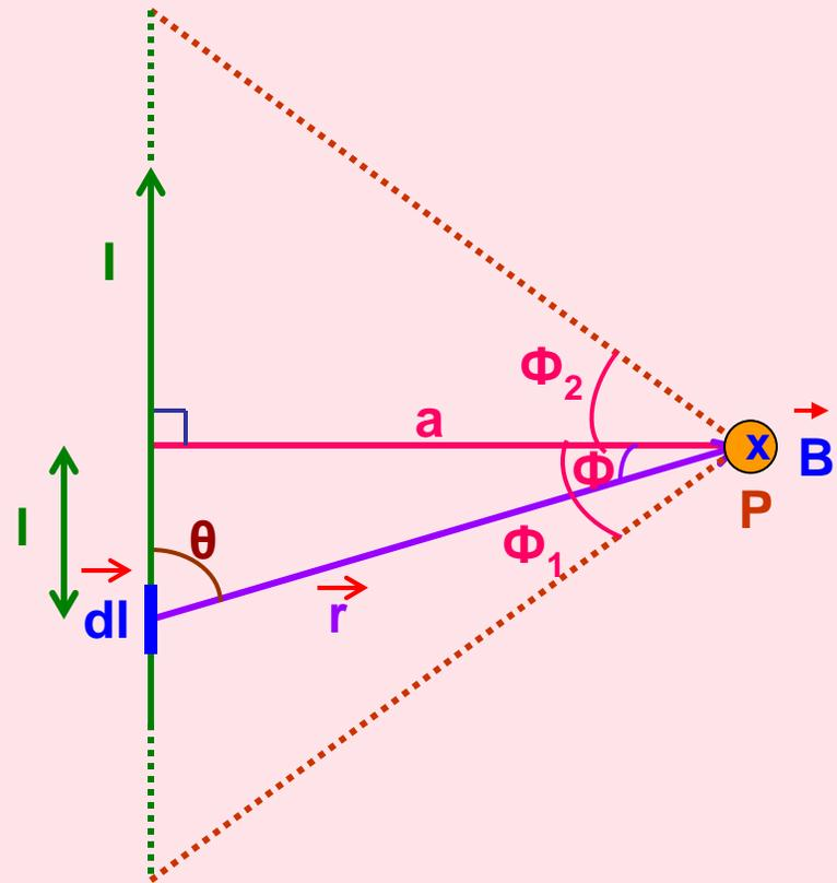
Magnetic field due to whole conductor is obtained by integrating with limits -  $\Phi_1$  to  $\Phi_2$ . ( $\Phi_1$  is taken negative since it is anticlockwise)
